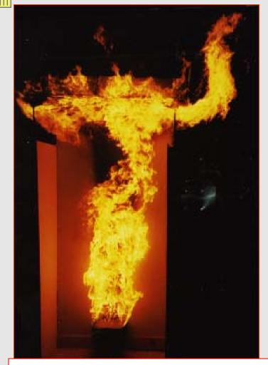
Burn through at a joint in a combustible (wood) soffit. This view is from the perspective of the attic.
