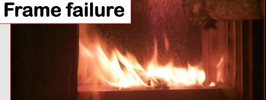
Horizontal separator on single- / double-hung window. (The horizontal separator in hung vinyl windows should be reinforced with an aluminum cross piece.)
